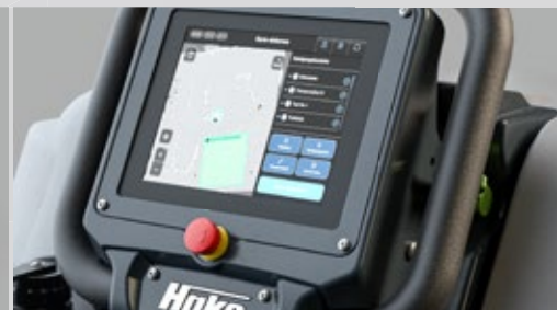
The 8-inch LCD panel clearly displays all relevant information.
