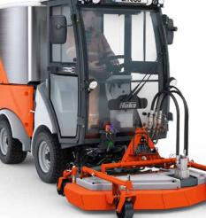
In combination with different mowers, grass collecting systems and flail mowers, the Citymaster 650 ensures flexible use for green area maintenance tasks in the gardening & landscaping sector. Together, the large universal hopper and the Citymaster 650 equipped with a mowing/suction attachment combi form a powerful team for efficient green area maintenance. Thanks to the central suction system, working close to kerbs and edges is possible on both sides of the machine.
