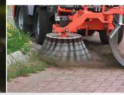
Weed control without the use of chemicals: with a weed broom providing fast and easy mechanical removal and collection of weeds.
