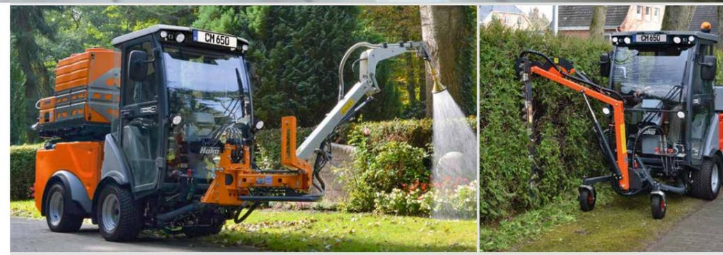
Weed control without the use of chemicals: with a weed broom providing fast and easy mechanical removal and collection of weeds.
